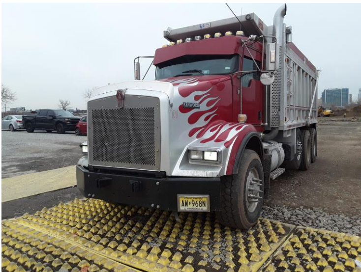
TRUCK LOADED WITH SOIL FOR DISPOSAL AND FODS PAD
