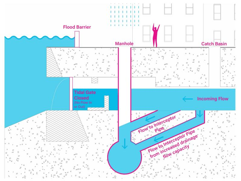
The proposed drainage system will allow additional flow capacity to the interceptor pipe, reducing the risk of street and basement flooding.
