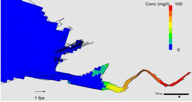
reopened, or, more simply stated, an in-water tidal barrier ABOVE: Coney Island Creek tracer model performed to illustrate water quality conditions within the Creek
