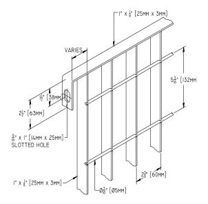
**30-INCH HT // 48-INCH HT METAL WIRE & BAR FENCE + GATES** Item: Maintenance Area Fence / **Grigliato Fence / Panel Type A** Manufacturer: **Metalco** or Approved Equal Material: **Galvanized Steel** Color / Finish: **Galvanized**
